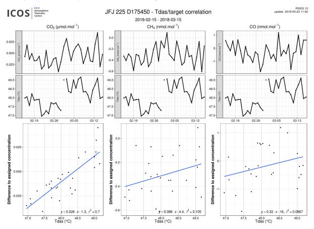
**General comments:** The temperature of the instrument is varying within 2°C. We do not detect any significant variability of the short-term target gas measurements with temperature for  $CO_2$ ,  $CH_4$  and CO.
