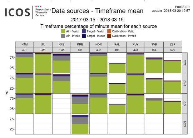
**General comments:** More than 90% of the data is air sampled from the mast. Only a few percent of data are dedicated to flushing, target or calibration sampling.
