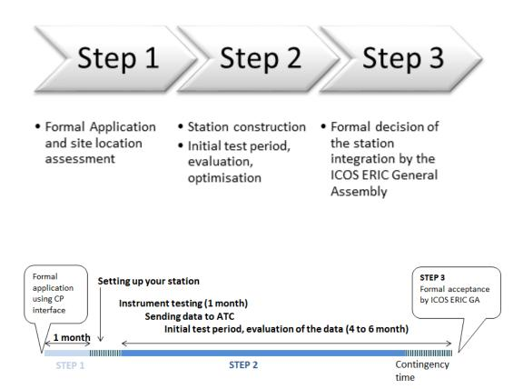
Once the data flow from the station to the ATC is in place, a phase of measurement optimization starts, the so called initial test period. This is done in close collaboration between the station PI and the ATC. This period typically lasts 4 to 6 months to gather enough time-statistics. The period can be prolonged if need be.
