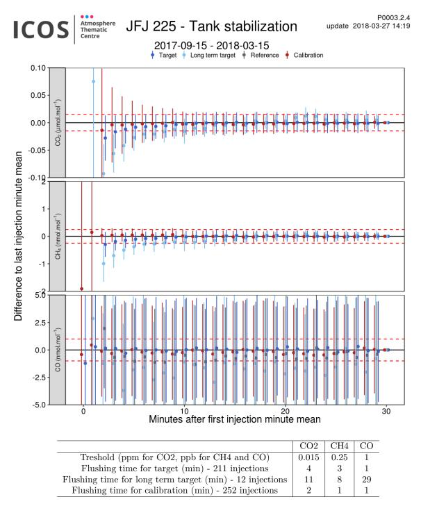
The flushing time is estimated as the time necessary for the difference between each injection and the last injection to be under the defined threshold. Thresholds are estimated relative to WMO goals and usual performances of instruments.
